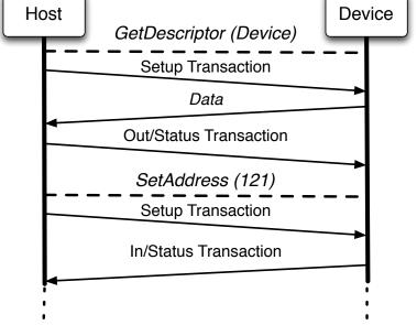
An example USB data flow. Control transfers (dotted lines) are comprised by a set of transactions (solid lines)
