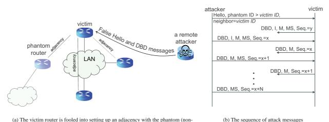
(a) The victim router is fooled into setting up an adjacency with the phantom (non-existent) router
