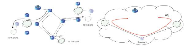
(a) Dashed lines show diverted traffic intended for the victim network (10.10.0.0/16). Traffic is diverted to the semitransparent phantom routers.
