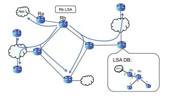
Figure 1. An example of LSA flooding
