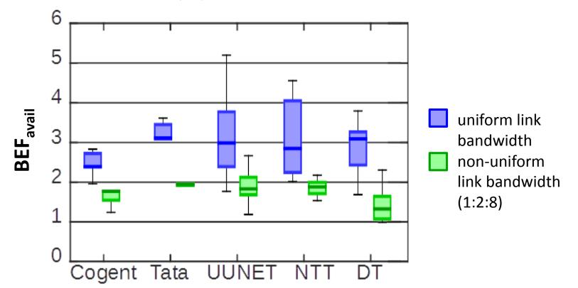
How to implement *TBE with large BEF<sub>ideal</sub> when BEF<sub>avail</sub> < BEF<sub>ideal</sub>?* ✓ randomized sequential TBE: we sequentially test only a random subset of senders at each TBE, providing them the ideal bandwidth expansion factor *BEF<sub>ideal</sub>*
