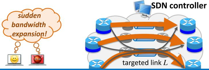
Linear programming formulation: We find the maximum available bandwidth expansion factor (BEF<sub>avail</sub>) and new routes for a target link and a given network topology
