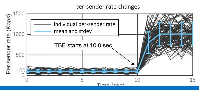
Large rate-change ratio can be quickly measured (e.g., < 5 sec)</li>
