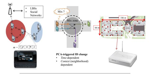
Figure 1. Left: System and network model with communities shown as shaded regions. Nokia N900 smart phone shown at bottom used in actual deployment. Middle: Mix-zone showing silent period and identifier changes. Right: Adversarial wireless mesh network of Asus routers.
