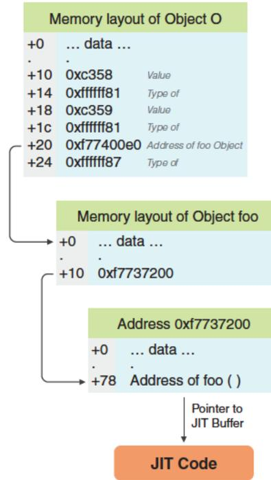
Fig. 7. The memory layout of Object `O` and Object `foo`, along with the necessary steps for locating a (code) pointer inside the JIT buffer. Once an address of the JIT buffer is known, all ROP gadgets can be discovered and the attacker can build the needed ROP chain for exploiting the browser.
