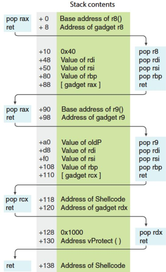
Fig. 6. The stack during the attack against IE.
