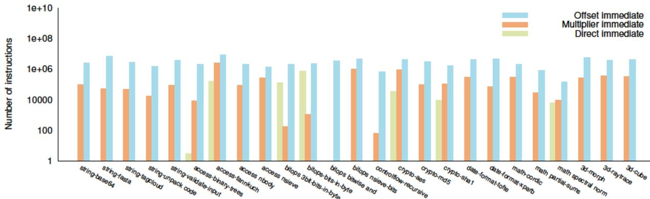
Fig. 9. Distribution of instructions emitted in the JIT buffer that affect an immediate value. There are basically three types of instructions that may involve an immediate value: *offset immediate* (e.g., `mov rcx, [rcx+0x8]`), *multiplier immediate* (e.g., `mov [r8+rdi*8+0x20], 0xffff88000`), and *direct immediate* (e.g., `shl r13, 3`).
