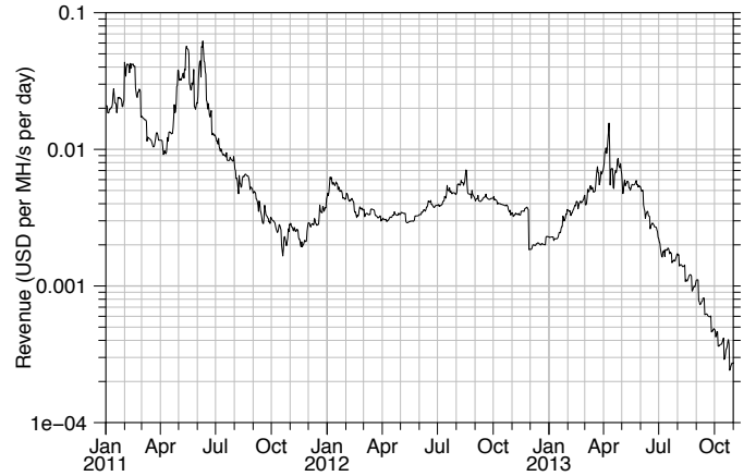
Fig. 9: Daily miner revenue per MH/s of mining capability. Daily revenue per MH/sec of hashing power is given by 86400 \cdot D \cdot U , where D is the expected revenue in BTC per million hashes computed, and U is the USD:BTC exchange rate.
