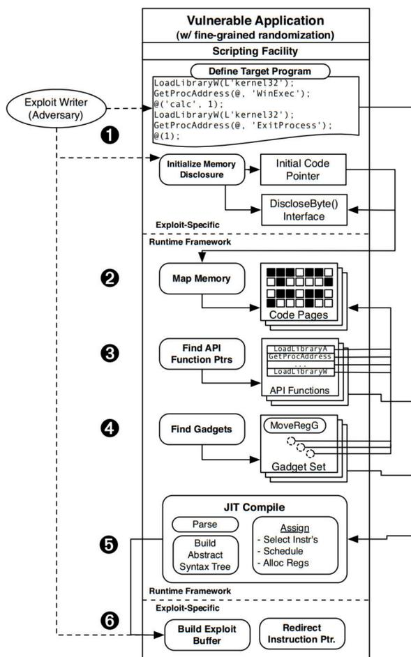
It should be noted that JIT-ROP attacks do not necessarily require a JIT compiler. Any exploit that finds and chains ROP gadgets on-the-fly can be considered as JIT-ROP. Since JIT-ROP requires (1) **memory disclosure**; and (2) **ROP gadget chaining**, we can mitigate it by restricting disclosed memory and raising the bar of chaining ROP gadgets, shown on the right.
