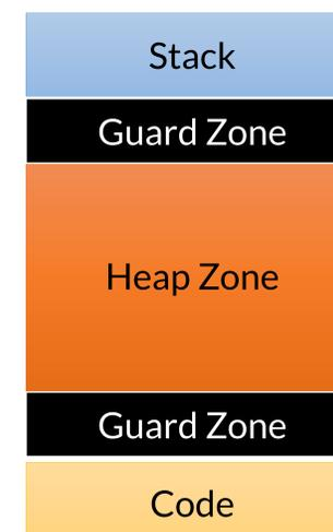
For each program, we allocate a heap zone in its address space that only holds program-allocated heap objects. No stack and code would be in the heap zone, therefore, any heap buffer overflow (sequential) or UAF will not directly steal or pollute information in the code and stack. For objects (e.g., JavaScript-accessible objects) that only operate on the heap, we can sanitize their access methods to make sure their access only happens in the Heap Zone.
