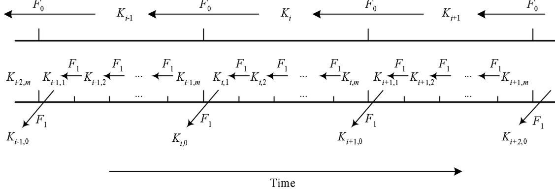
Figure 1. The two levels of key chains in Scheme II. Each key  $K_i$  is used for the high-level time interval  $I_i$ , and each key  $K_{i,j}$  is used for the low-level time interval  $I_{i,j}$ .  $F_0$  and  $F_1$  are different pseudo random functions. Each commitment  $K_{i,0}$  is distributed during the time interval  $I_{i-1}$ .
