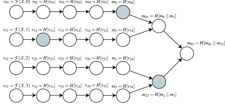
**Figure 5:** Example tree-authenticated one-way chain construction for authenticating a sequence of one-way chains. The instance in this figure allows 4 sequence numbers to be authenticated, and metrics up to 3. The shaded values represent sequence number 1 metric 1.
