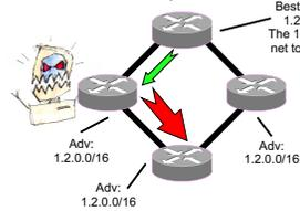
Reactors hole-punch routes adding blacklisted ASes, loop detection prevents route propagation
