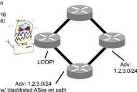
BGP will forward using the hole-punched route if available, which will not traverse over attacked links
