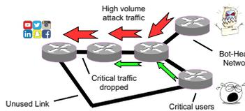
Our system can manipulate routes so that critical traffic stays off attacked links while other links are under stress due to an attack
