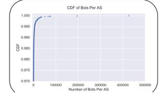
If we can move legitimate, non-bot traffic off the links that are along the best paths for those ASes, then we can halt the effects of DDoS attacks since there are a small number of ASes with a large amounts of bots
