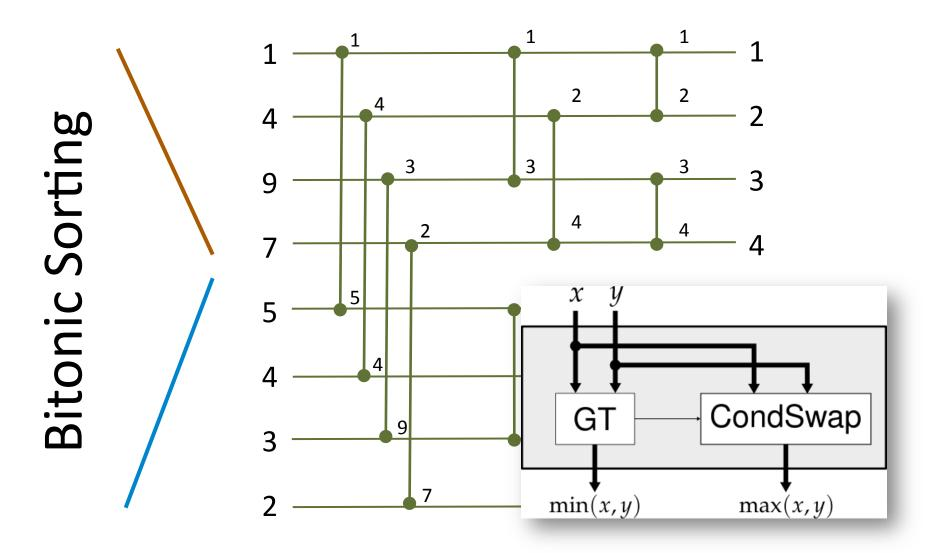
Sort 2n bitonic inputs with  $n \log(2n)$  CompareSwap circuits.
