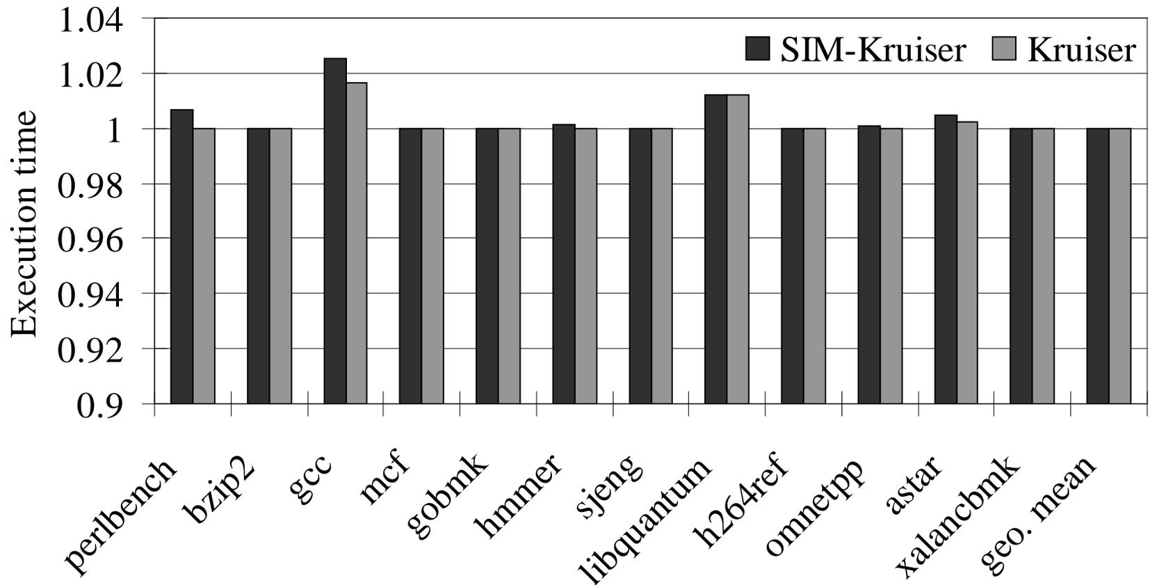
SPEC CPU2006 performance (normalized to the execution time of original Linux).
