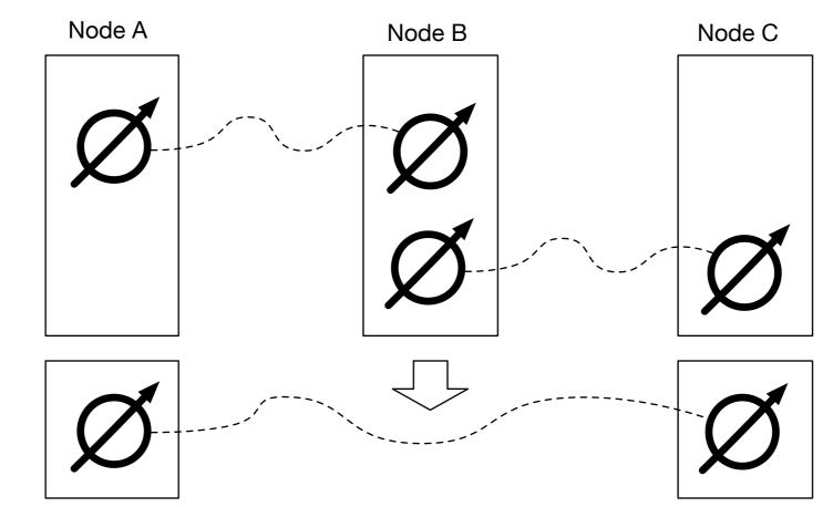
After entanglement swapping, qubits in the middle node does not provide any role, can be reused
