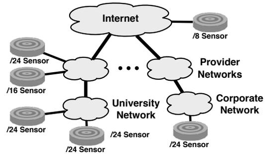
Figure 1. Internet Motion Sensor Architecture
