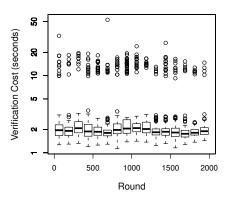
Figure 5. Verification cost per round using eager round constraints and *XPilot*-specific optimizations, while checking a 2,000-round *XPilot* game log
