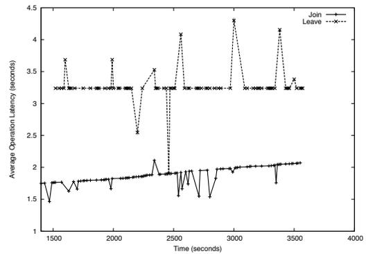
**Figure 10. Combining the optimizations of increased processors and increased content cryptosystem attributes in the satellite radio model allows operations to be bounded by tight latency requirements.**
