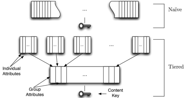
**Figure 3. A comparison of the naïve and tiered constructions for providing efficient access to content keys. Because join and leave operations can be performed on groups, the tiered construction is more efficient.**
