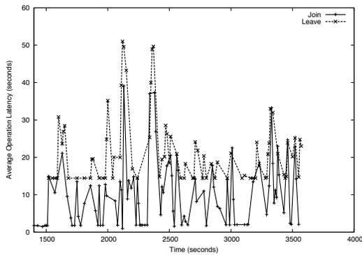
**Figure 9. Increasing the size of  $n'$ , the number of attributes in the content cryptosystem, reduces peak latency from minutes to seconds in the satellite radio model while incurring a nominal increase in decryption costs.**
