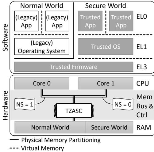
Figure 1: TrustZone software and hardware components. Software can be executed in *normal world* or in *secure world*. Isolation between these two worlds is enforced by the memory controller (TZASC) that checks for each memory access which world it originates from.
