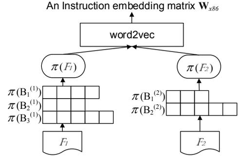
Fig. 3: Learning instruction embeddings for x86.  $\pi(\mathbb{B}_i^{(j)})$  represents the  $i$ -th block-level instruction stream (BIS) in the function  $\mathbb{F}_j$ . Each square in a BIS represents an instruction.
