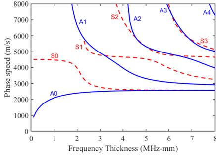
Fig. 3: The phase-velocity dispersion curve of a glass table.
