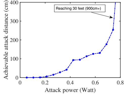
Fig. 14: Relationship between attack power and distance.
