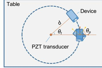
Fig. 12: An illustration of the directionality evaluation.
