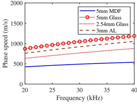
Fig. 15: The phase-velocity dispersion curves of A0 mode in different tables at the attack frequency range.
