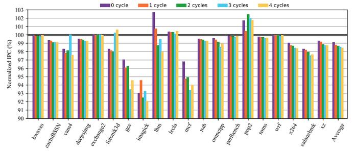
Fig. 11. Impact of calculation latency on PhantomCache performance.
