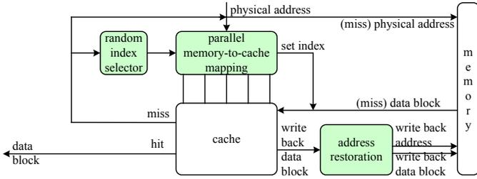
Fig. 4. PhantomCache architecture.
