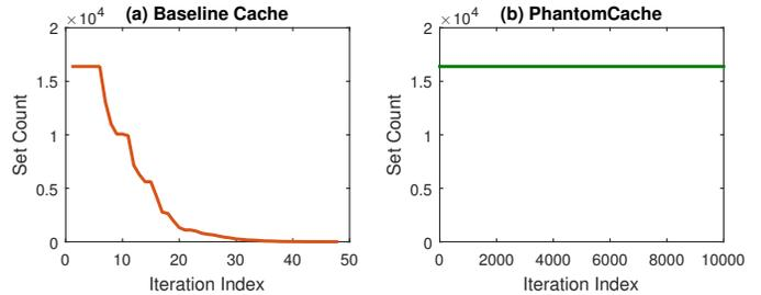
Fig. 9. Comparison of resistance to eviction set minimization.
