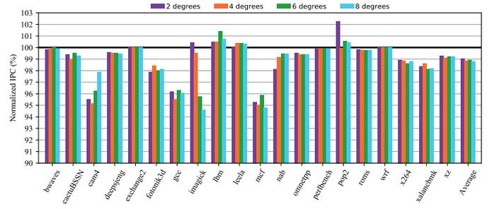
Fig. 12. Impact of randomization degree on PhantomCache performance.
