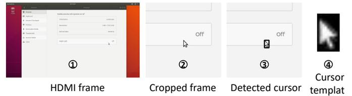
Fig. 13: **Cursor detection on the HDMI frame.** The figure shows PROTECTION mouse pointer tracking. ① shows the captured HDMI frame captured by B101 HDMI to CSI bridge. ② shows the cropped HDMI frame based on the mouse position received by the IOHUB. ③ shows the detected mouse pointer. For testing, we program the IOHUB to put a rectangle around the pointer. ④ shows one of the pointer templates that we used in our OpenCV routine.
