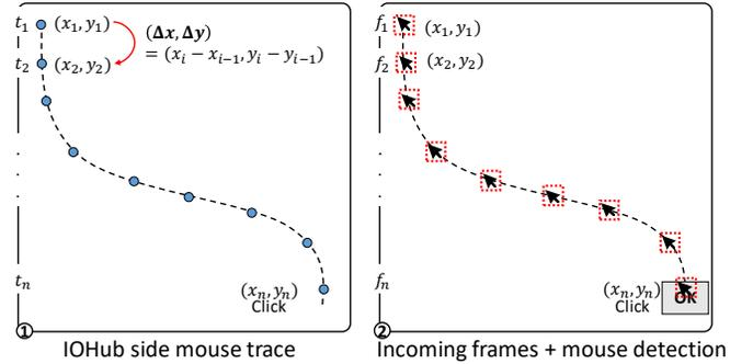
Fig. 6: **Pointer tracking.** ① The IOHUB captures the raw mouse events  $(\Delta x, \Delta y)$  from the mouse that is attached to the IOHUB. ② The IOHUB captures the frames from the HDMI channel and checks into the designated pixel position  $(x_i + \Delta x, y_i + \Delta y)$  if there exists a pointer.  $t_1, t_2, \dots, t_n$  are the time instances when the IOHUB receives the mouse data.  $f_1, f_2, \dots, f_n$  are the corresponding HDMI frames that the IOHUB intercepts.
