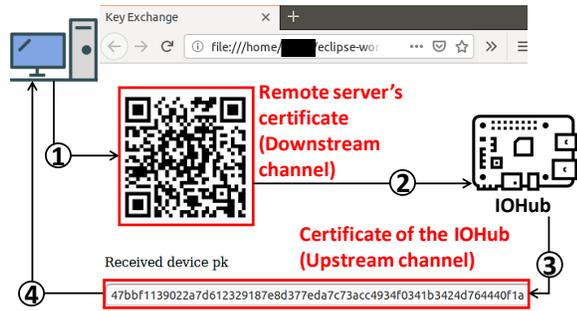
Fig. 12: **Establishing TLS.** A snapshot of the key exchange web page that is used to communicate the public certificates of the device and the remote server.
