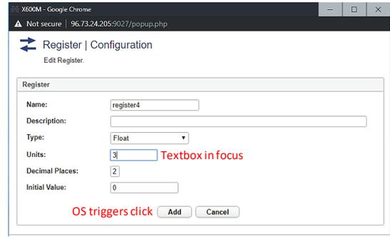
Fig. 2: Early form submission attack is possible on Fidelius [9]. The user selects and edits the field `Units` while the OS triggers add button, causing misconfiguration of a remote safety-critical PLC (Control by Web X-600M [1]).
