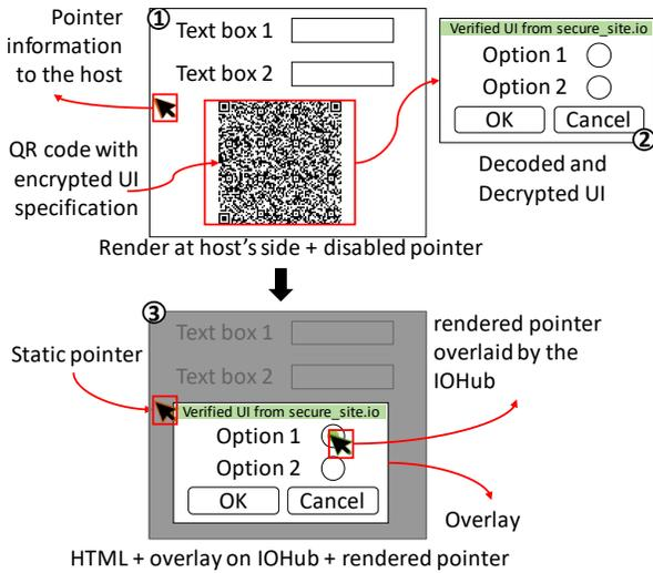
Fig. 8: **PROTECTION IO confidentiality.** The figure shows ① the browser render of the webpage in Specification 2 where the PROTECTION JavaScript produces the encrypted QR code. ② shows the UI overlay that is decrypted and decoded by the IOHUB. ③ shows the user's view when the IOHUB overlays the UI on the HDMI frame, and the user starts to interact with the UI.
