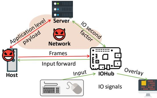
Fig. 3: **High-level approach overview of our solution.** The IOHUB connects the trusted IO devices and the attacker-controlled host.
