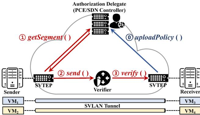
Fig. 2: High-level overview of SVLAN.
