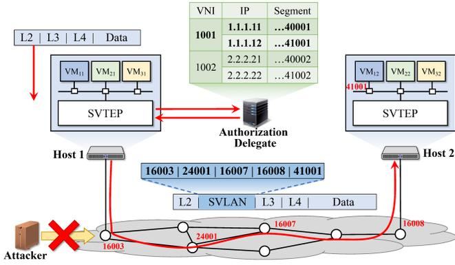
Fig. 3: Only authorized senders can retrieve valid path segments and forward packets to the receiver.
