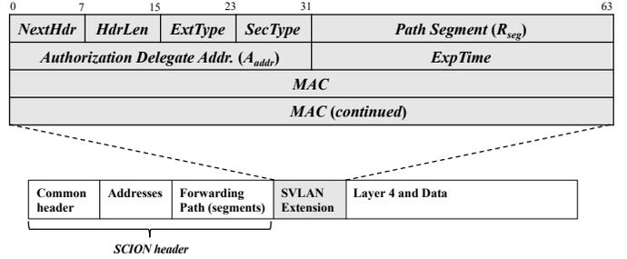
Fig. 4: The header format of the SVLAN extension.
