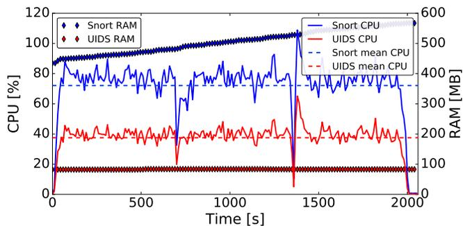
Fig. 4. UIDS vs. Snort — Port scan (TRAbID, LAP).
