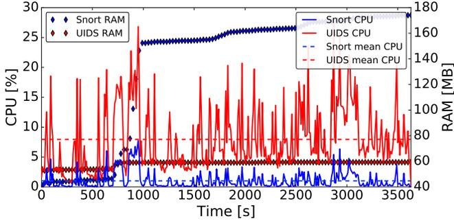
Fig. 8. UIDS vs. Snort — Port scan (CICIDS2017, RPI).
