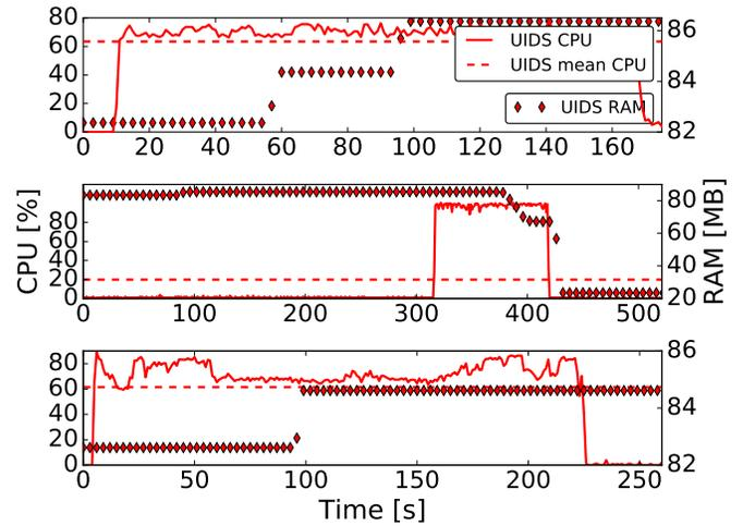
Fig. 10. UIDS stress-test (LAP) — Saturated 1Gbps link (top). Background traffic plus attacks (middle). 1Gbps, 5000 concurrent TCP connections (bottom).
