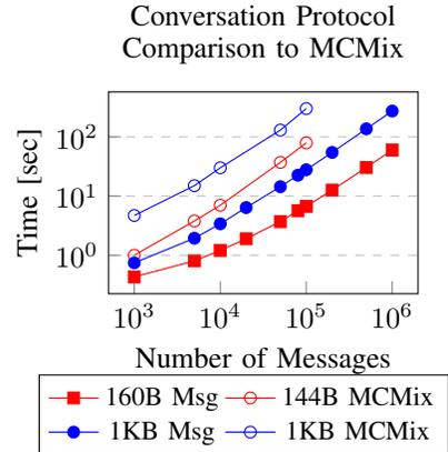
Fig. 4: Performance of our messaging conversation protocol for various message sizes compared to MCMix [3]. For 100,000 160 Byte messages, our scheme shuffles the messages 11.8 $\times$  faster than MCMix.
