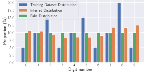
Fig. 16: Mitigation performance. The blue bar shows the original distribution of each digit in the training dataset, while the orange one depicts the inferred distribution based on our full black-box attack. The green bar shows the fake distribution after rebalancing dataset.
