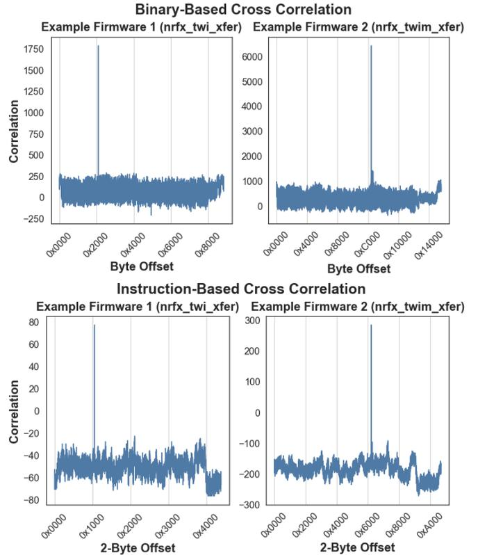
Fig. 4: Cross Correlations of Function Binaries and Instructions for 2 firmware examples using different library functions for I2C communication. The correct byte offset should be `0x21AC` and `0xC6E4` in firmware 1 and firmware 2 respectively.
