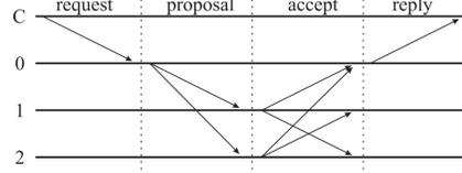
Fig. 6: Diagram of a normal case SMR operation (from [33])
