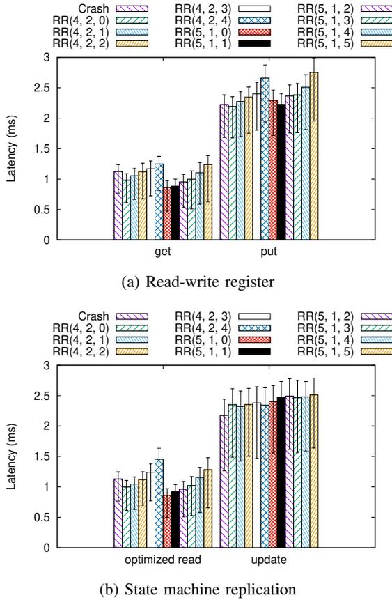
Fig. 11: Latency for different configurations and models in the 1ms topology. CFT uses  $F = 3$  and  $RR(M_R, F, s)$  denote RR with parameters  $M_R$  and  $F$ , with  $s$  restarts.
