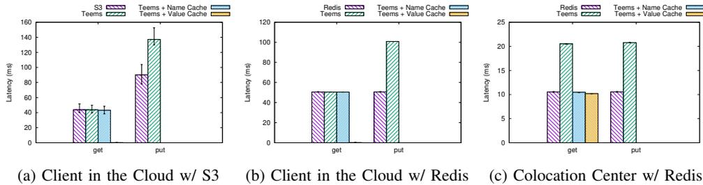
Fig. 12: Latency in different deployment scenarios. The “s3” and “redis” bars refer to direct accesses to the untrusted storage, providing a performance baseline without rollback protection. “teems” refers to accesses without caching. “teems + name cache” and “teems + blob cache” refer to accesses where the name and blob caches had a hit, respectively.
