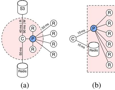
Fig. 8: Deployment scenarios: (a) cloud client, (b) colocation center. The shaded area represents a LAN (or a data center). Latencies will be used in the evaluation.  $C$  is the client,  $R$  is a replica and  $P$  is the proxy replica.
