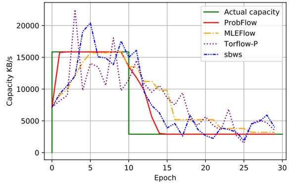
Fig. 10: Exit relay joining after 10 epochs having an actual capacity of 15851 KB/s then changing capacity after 10 epochs to 2898 KB/s.
