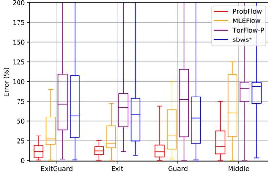
Fig. 8: Relays capacity estimation error distribution using the 4 different algorithms in fully utilized network scenario after 20 epochs computed for the 5 sample of a 3% network.
