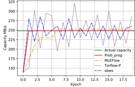
Fig. 5: The estimated capacity of an exit relay joining the network after 10 measurement epochs and staying for 20 epochs in MB/s.
