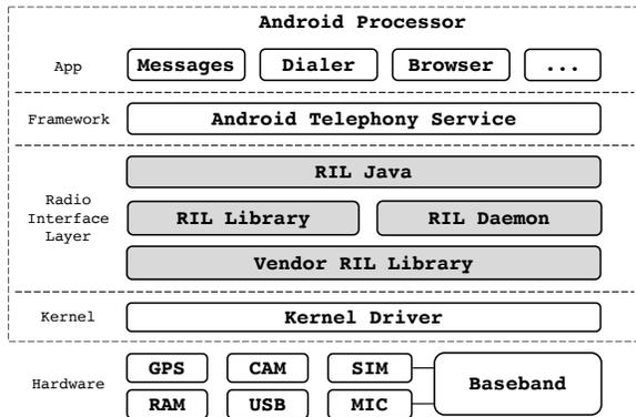
Fig. 3: Typical architecture of an Android UE.
