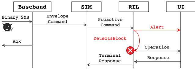
Fig. 5: Interactive binary SMS detection and mitigation.
