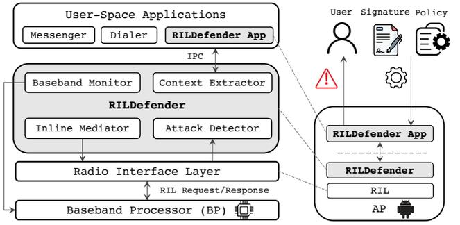
Fig. 4: A high-level illustration of RILDEFENDER.
