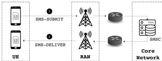
Fig. 1: SMS transmission path in a cellular network.
