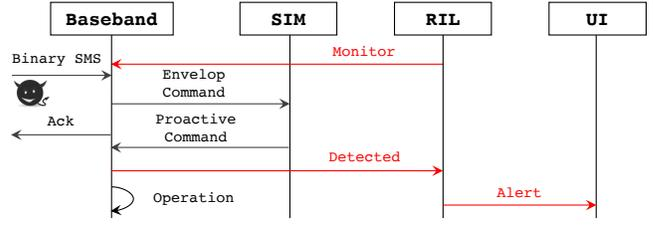
Fig. 6: Non-interactive binary SMS detection and mitigation.
