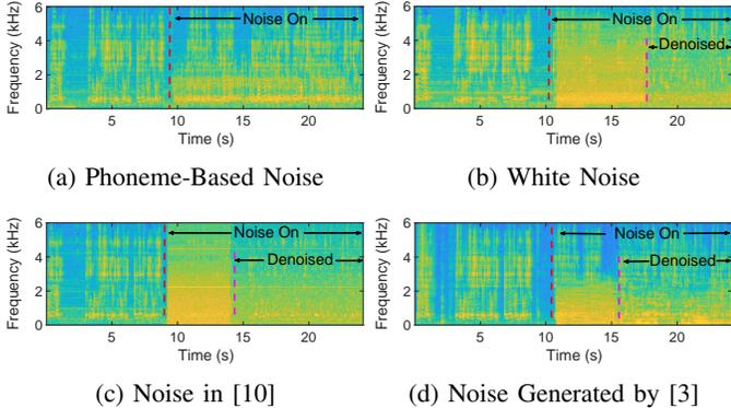
Fig. 7: Comparison of the robustness of different noises against the built-in noise reduction in a Vivo Nex smartphone.
