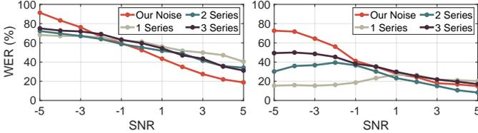
Fig. 22: Comparisons with speech-like noise. Left: WER before noise reduction. Right: WER after noise reduction.
