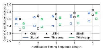
Fig. 8: Overall classification accuracy (y-axis) for the receiver classification per country, depending on delivery notification timing sequence length (x-axis) and NN type (icon shape)
