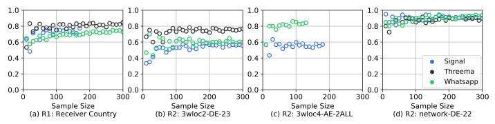
Fig. 12: Overall accuracy of four different classification tasks, depending on the number of samples per class (x-axis).
