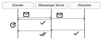
Fig. 3: Schematic overview of the message flow from the senders' perspective. The illustration is simplified since sender and receiver can be connected to different messenger servers.
