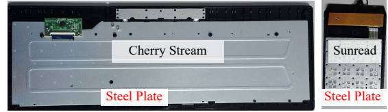
Fig. 25: Illustrations of the steel plate underneath the matrix circuit, which shields the matrix circuit from GhostType attack.
