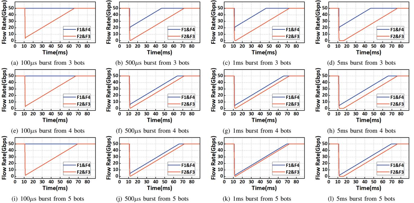
Fig. 2. Flow rate with different burst duration  $\tau$  and peak rate  $\delta$ .
