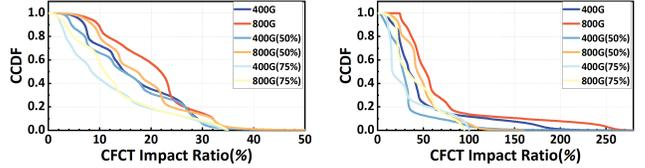
(c) Co-flow completion time impact ratio of distributed machine learning training with a high flow number. (d) Co-flow completion time impact ratio of cloud storage with a high flow number.
