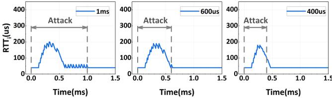
Fig. 6.  $RTT_i$  variation with different burst duration.
