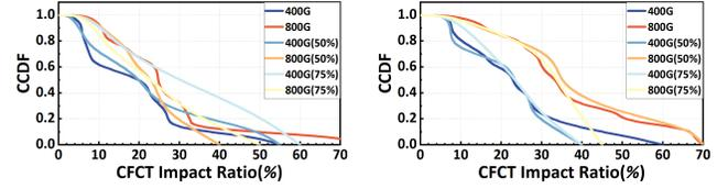
(a) Co-flow completion time impact ratio of distributed machine learning training with a low flow number. (b) Co-flow completion time impact ratio of cloud storage with a low flow number.
