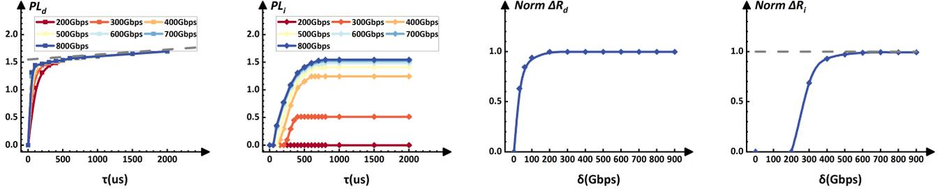
(a) Performance loss on direct victim flows  $PL_d$  with burst duration  $\tau$ . (b) Performance loss on indirect victim flows  $PL_i$  with burst duration  $\tau$ . (c) Normalized performance loss factor  $\text{Norm } \Delta R_d$  on direct victim flows with burst peak rate  $\delta$  ( $\tau = 1ms$ ). (d) Normalized performance loss factor  $\text{Norm } \Delta R_i$  on indirect victim flows with burst peak rate  $\delta$  ( $\tau = 1ms$ ).
