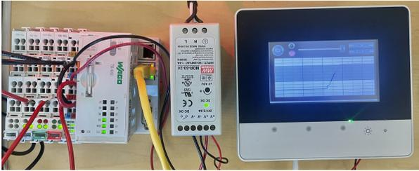
Fig. 5: PLC, Power Supply, and Microbrowser HMI
