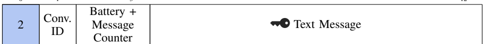
(b) Emergency text message sent during an emergency conversation. The maximum text message length is 160 byte.
