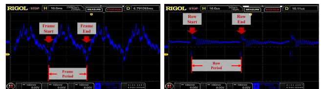
Fig. 17: The electromagnetic leakage of target camera recorded at (a) 10ms and (b) 16 $\mu$ s per cell.
