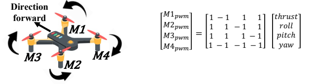
(a) A quadcopter hovering in the air, (b) Mixer algorithm for adjusting motor thrust.
