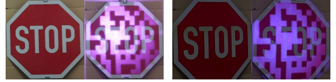
(a) Raspberry Pi Camera 3 (b) Leopard Imaging AR023ZWDR Fig. 12. Infrared perturbation captured with two different camera sensors.
