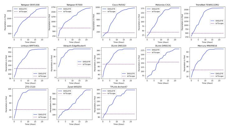
Compared with IoTScope, EAGLEYE can not only obtain more parameters but also the parameters are more accurate. To a certain extent, this trend reflects the continuous improvement of EAGLEYE's mutation quality with the continuous supplement of parameters from responses.
