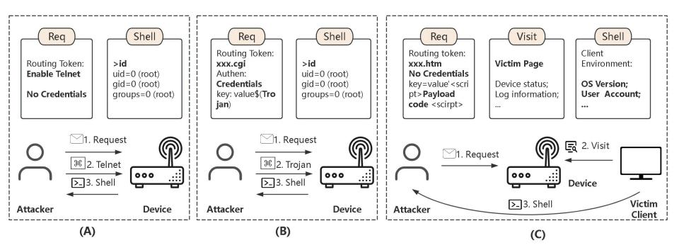
Three typical vulnerabilities in discovered hidden interfaces. (A) A backdoor bypassing authentication: opens the telnet and gains a shell with the highest privilege. (B) A command injection escalating privilege: allows attackers with normal credentials to execute OS commands with the highest privilege. (C) An XSS attacking victim's clients: injects malicious code into one parameter saved in the web, and then the users who visit the victim pages will be infected.
