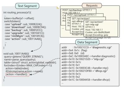
(a) An illustrative program demonstrating a specific routing process that incorporates two-level routing tokens, distinctly positioned within the URI and the query string.
