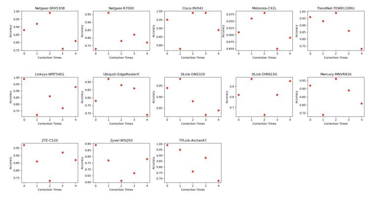
Accuracy of the pattern learned by LLM varies with the number of corrections. Within limited adjustments, the LLM can learn the correct features among the routing table.
