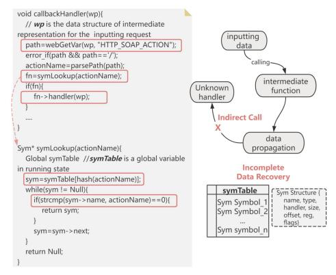
Data flow along the interface is hard to trace, due to some open problems like indirect calls and incomplete data recovery.
