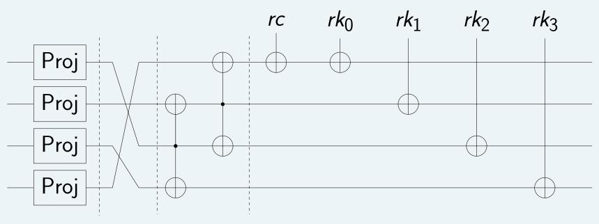
Permutation layer Round constant/Key addition layer Substitution layer Mixing layer
