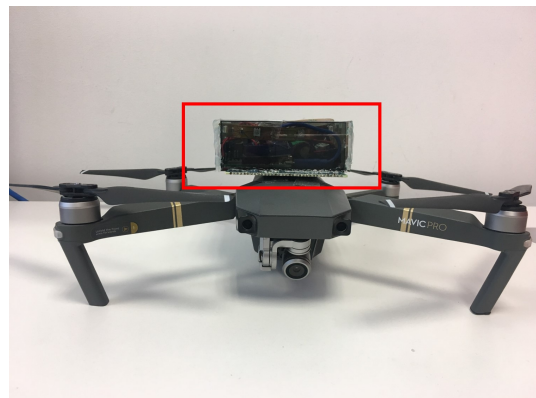
Fig. 2. The authenticating device mounted on a drone to transmit message.
