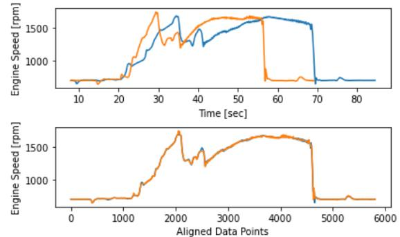
Fig. 1. Engine speed traces for Cycles A and B, showing pre-alignment (top) and after application of DTW (bottom).
