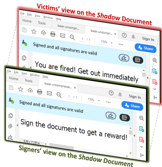
Figure 1. A shadow PDF document presents a trustworthy content to the signers (top document). After signing this document, the attackers modify the document and enforce another view of the document on victims' side without invalidating the signature (bottom document).
