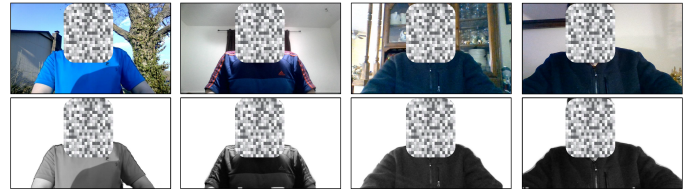
Fig. 17: Example output of the background removal process, using DeepLabv3 and Microsoft COCO, successfully applied in different indoor and outdoor settings. Top four images are the original frames, and bottom four images are corresponding frames after background removal.
