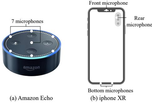
Fig. 3. Modern smart devices support multiple microphone to obtain high-quality audio. The microphone array of Amazon Echo (7 microphones) [21] and iPhone XR (4 microphones) [18].
