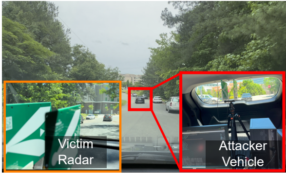
Fig. 17: Experimental setup for the moving vehicles studies.
