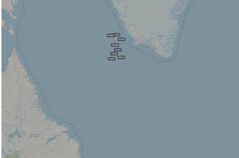
(b) Fake position of aircraft after injecting malicious ADS-C reports into our setup.
