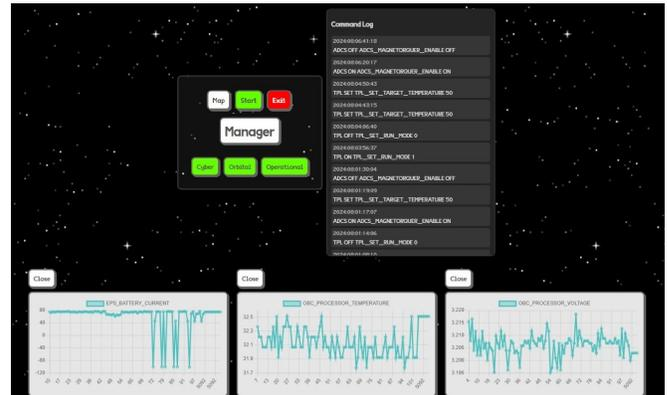
Fig. 3. The simulation manager component’s web application, which incorporates live data visualization, including graphs of telemetry data and command logs, and facilitates real-time monitoring of the primary components and the scenario’s execution.
