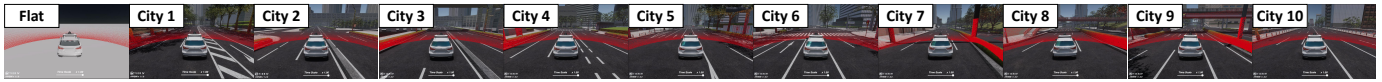
Fig. 7. LiDAR point cloud measurement in AWSIM simulation for each scene. The red points represent the point cloud measured by LiDAR.
